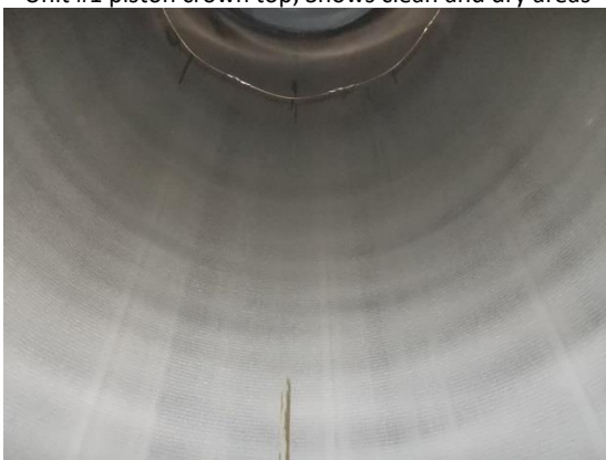
Unit #1 piston crown top; Shows clean and dry areas
