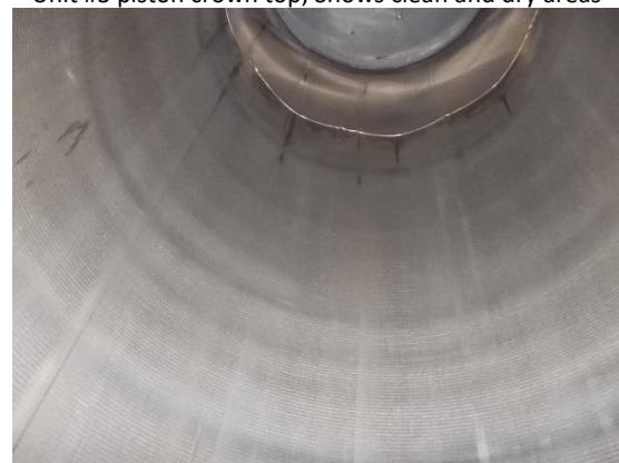
Unit #3 piston crown top; Shows clean and dry areas
