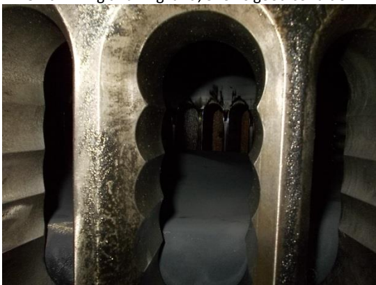
Unit #1 piston crown top; Shows clean and dry areas
